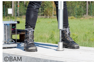
©BAM Vibration test. Hammer hit by free-drop weight.
