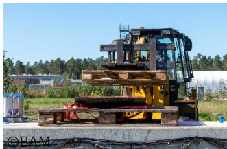
©BAM Loading test. Various loads by iron bars: 300, 600, 900 kg.
