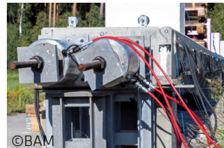
©BAM Pressing test. Built-in post-tensioning system.
